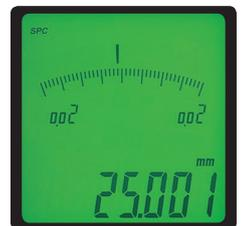
Difference / runout measurement
