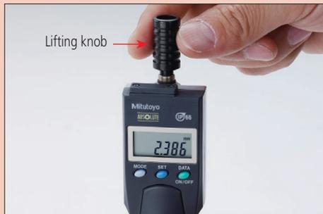
Plunger can be manually lifted. Remove the plunger cap for ID-N and attach the lifting knob to the plunger. Note that water resistance is not maintained in this configuration.
