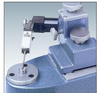
Calibrating a lever probe head.
